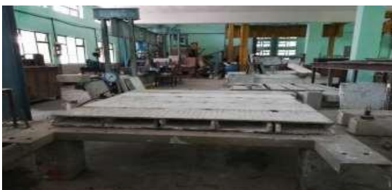
Fig. 7 Typical Closed Channel Slab
