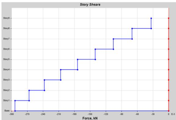
Graph 3 storey shear curve for isolated base structure
