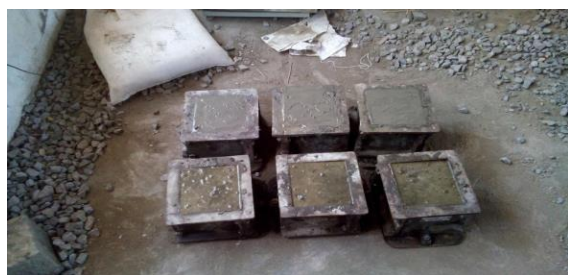
Figure 3: Casting of Specimens
