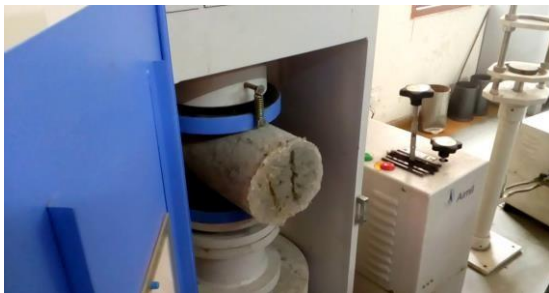
Figure 11: Test setup for Split Tensile Test
