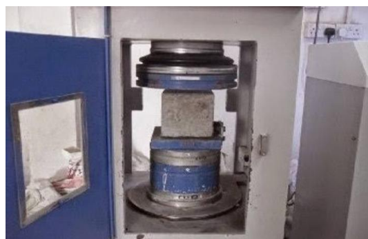
Figure 5: Test setup for the compressive strength
