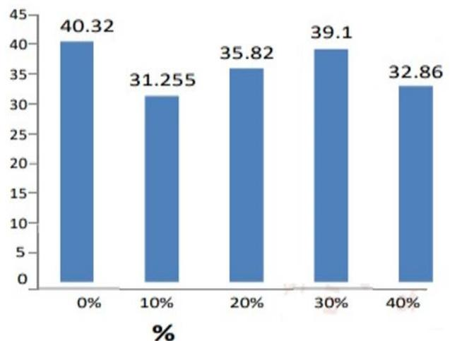
Figure 3: Graph between percentage of fine aggregate replacement and respective Split Tensile strength of the plastic replaced concrete
