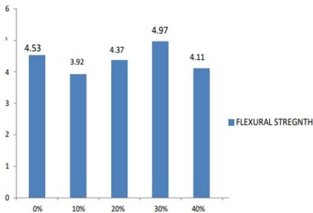
Figure 2: Graph between percentage of fine aggregate replacement and respective Flexural strength of the plastic replaced concrete
