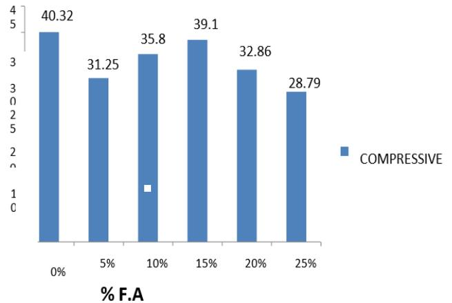
Figure 1: Graph between percentage of fine aggregate replacement and respective compressive strength of the plastic replaced concrete
