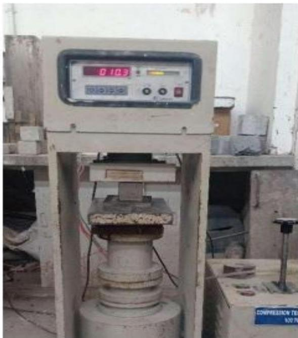
Figure 4: Compressive strength of mortar
