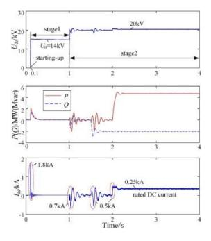
Figure 5: wave forms during starting.
