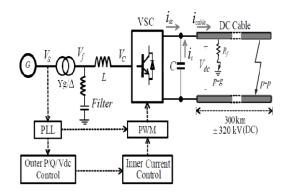
Figure 3: HVDC With two level Inverter.
