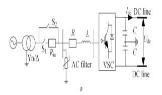
Figure 6: Starting circuit of HVDC
