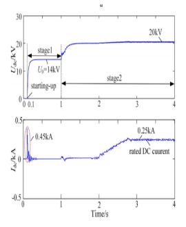
Figure 10: Changes In Current And Voltage.
