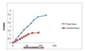
Graph 1 Push over curve for both the fixed and rubber isolated base
