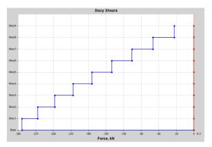
Graph 3 storey shear curve for isolated base structure
