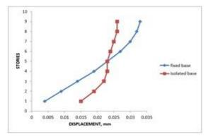
Graph 2 Displacement curve for all the stories for both fixed and rubber isolated bases
