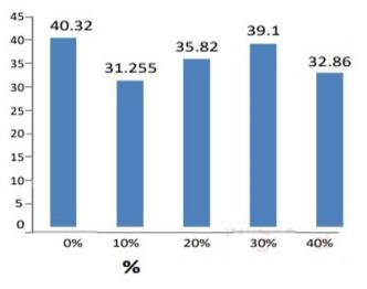
Figure 3: Graph between percentage of fine aggregate replacement and respective Split Tensile strength of the plastic replaced concrete
