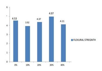
Figure 2: Graph between percentage of fine aggregate replacement and respective Flexural strength of the plastic replaced concrete
