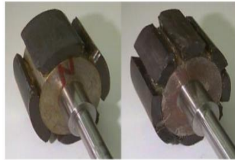
Figure 7: 4 pole/ 8 pole rotor.
