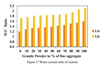
The rough and angular texture of GP (refer SEM in Figure 3.7) was reason behind this increment in water-cement ratio. Due to such texture of GP resistance to flow of mortar was increased which required more water to attain required flow. The greater water absorption by GP as compared to FS may also be another reason for increment in water demand.
